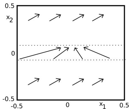
**Figure 4.** A Soft-synchronized oscillator pair as a dynamical system whose phase space is a torus. Inside the region between the two dotted lines the phase of the first oscillator is pushed toward zero.
