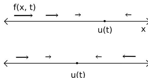
**Figure 1.** Low-pass filter considered as a dynamical system. The input,  $u(t)$ , varies with time, and as a result the vector field that defines the dynamical system does also. The vector field also depends on the roll-off frequency of the filter.
