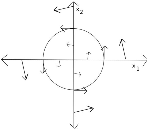
**Figure 2.** A sinusoidal oscillator realized as a two-dimensional dynamical system. The circular path is the limit cycle of the oscillator. Points that do not lie on the circle (except the origin) spiral inward or outward to the limit cycle.
