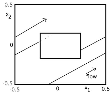
**Figure 5.** A phase space with a rectangular wormhole in the shape of a rectangle. The vector field is uniform, but whenever the state would enter the wormhole, instead it jumps to the diametrically opposite point.
