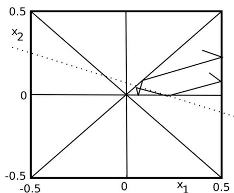
**Figure 6.** A Soft-synchronized oscillator pair as a dynamical system whose phase space is a torus. The dotted line shows the path through phase space and the solid line shows the corresponding path through one of the triangles.
