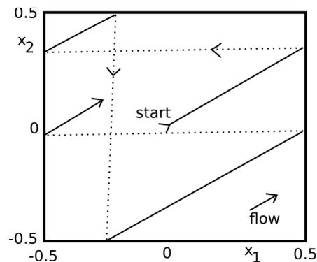
**Figure 3.** Phase space representation of a pair of uncoupled oscillators. Each phase ranges from -0.5 to 0.5. The vector field (the “flow” is uniform. Its two components are the frequencies of the oscillators.
